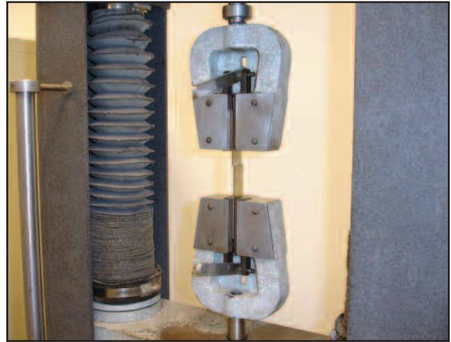
The lap shear testing machine in one of PSI's laboratories. Results are graphed by computer.
