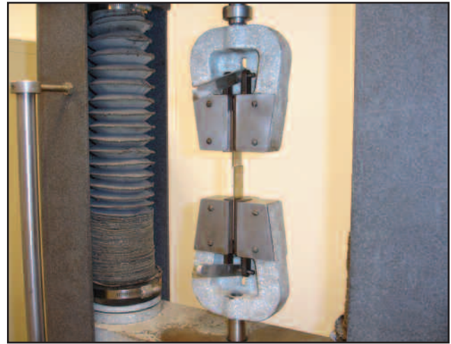
The lap shear testing machine in one of PSI's laboratories. Results are graphed by computer.
