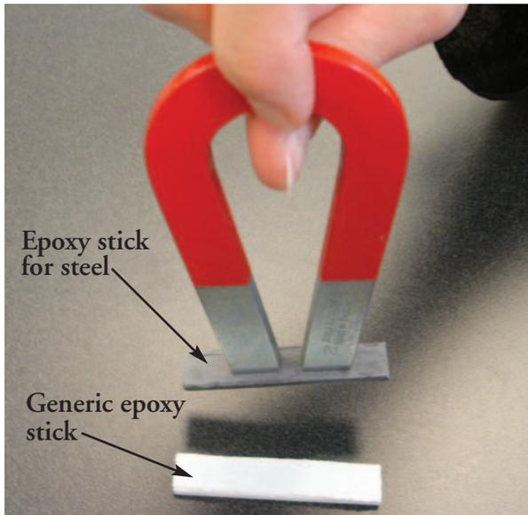
*The epoxy stick designed for steel actually contains steel, so an ordinary magnet picks it up. The generic epoxy stick has no steel, so it is not only less strong but cannot recognize the magnetic force.*
