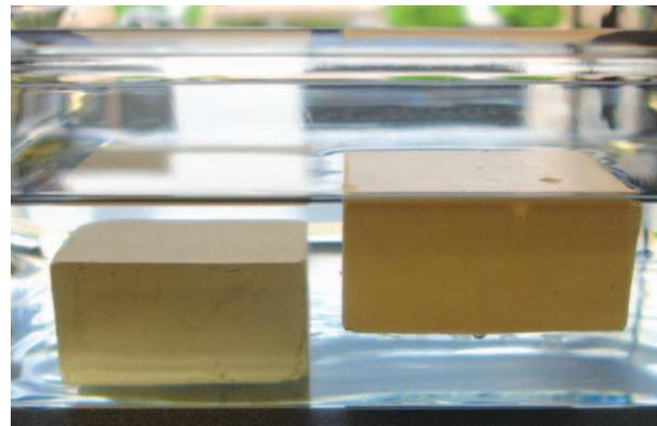
*The best epoxy sticks are designed for specific end uses. Here the generic epoxy stick sinks to the bottom, while the stick made specifically to repair wood actually floats.*
